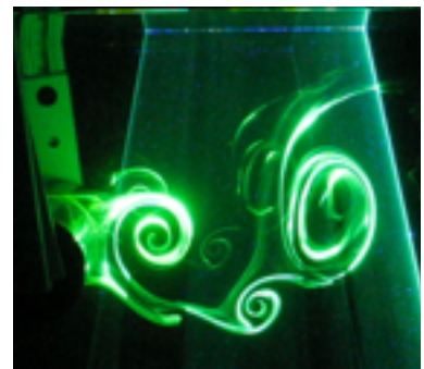
Dye flow visualization of vortices rolling up downstream of a cylinder. The dye is illuminated by a green planar laser sheet.
